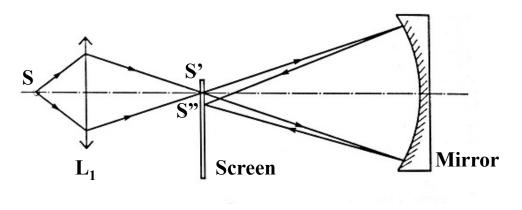
Figure 4: Measurement of radius of curvature of a concave mirror
