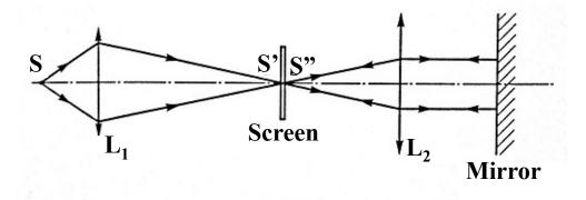
Figure 5: Measurement of the focal length of a lens by an autocollimation method
