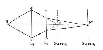
Figure 2: Measurement of the focal length of the diverging lens
